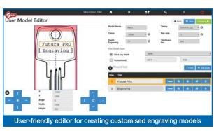
for just as many Silca references (keys, medals and plates), which identify the areas for inserting the text you want to engrave. For each reference, you can select the depth of the incision, whilst the software indicates the jaw step you should use.
