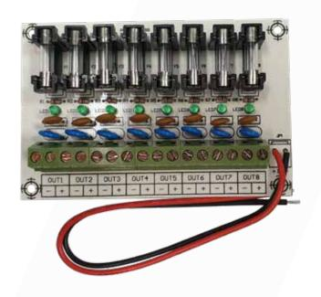
Power supply Module, 8 x 500mA Individually Fused Outputs suit NEPSDC5A01B
